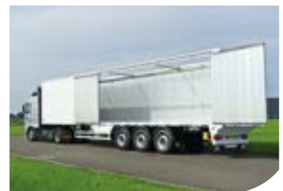
Self-supporting construction with side doors
