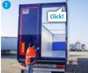
Swing the upper beam back into its locking device.
