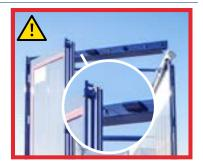
Only release the upper beam when the cam lock is in the second position as described in step 3.
