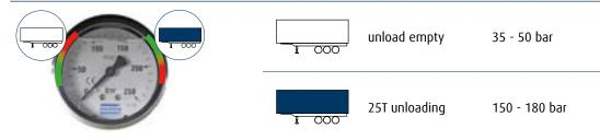
The difference in oil pressure can be seen when all floor planks move simultaneously or when only 1 group moves.
