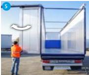
Use the sheet stick to pull down the Swing the left door open. The trailer is now ready for use.
