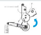
Tighten the wing nut well and use the rotation block to prevent the tube from turning while driving.
