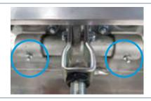
Lubricate with a grease gun.
