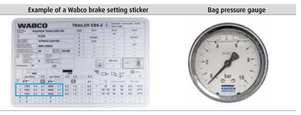
Indication of the pressure in the bags with corresponding weights. This depends on the type of axle and air bags. The settings can be found on the Wabco sticker. For position see Ch 2.1
