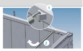
Lift the bar out of the block, turn the bar towards the holder and replace the locking pin. Never turn away all the bars at the same time.
