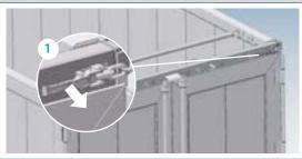
Unlock the locking device on the underside.
