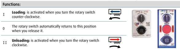
For safety, this switch is equipped with an automatic spring return for positions I and II, so that it always returns to the centre "0" position. This is necessary to prevent a functioning that conflicts with the CF8 remote control.
