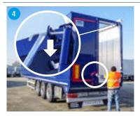
locking devices on the upper beam. Pull open the left rear door at the same time.
