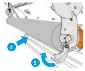
When closing the tube holders, the rotation block must remain open so that the roll-up sheet can turn (6).
