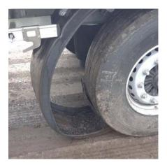
The following tips can help you easily prevent the spray protectors and mudguard being pulled off.
