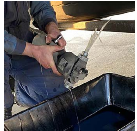
Residues of filter material in the hydraulic system
