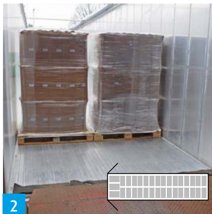
2 For a maximum load, position the pallets transversaly, and two side-by-side in the width of the trailer.
