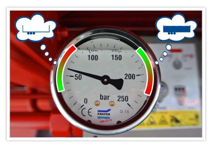
Knapen Trailers supplies a pressure gauge as standard with every new trailer. If you do not yet have a pressure gauge on your moving-floor trailer, your dealer sells separate pressure gauges that are easy to fit yourself. They fit every CF500-SL2 system and can be ordered using part number BHYCO10329. If you use this number, you will automatically order the hydraulic connector too. This will enable you to fit the pressure gauge directly to your Cargo Floor.
