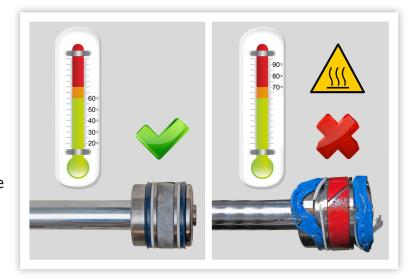
A high outside temperature obviously greatly aggravates the above factors. On the photo above you can see what can happen without a temperature safety device. If you want to be able to unload and minimise the chance of your seals melting, then a temperature safety device is a good option.
