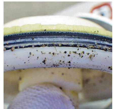
Result: As a result of contamination in the air hoses, the inside of the EBS modulator also becomes contaminated.
