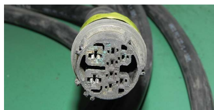
Result: if the union nut is poorly tightened, moisture can enter the cables leading to corrosion
