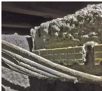
Regularly clean the EBS modulator and the cabling
