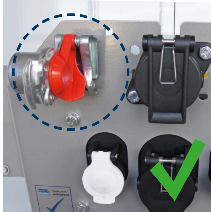
Always close the covers on the hose couplings so that no contaminants can enter the hoses
