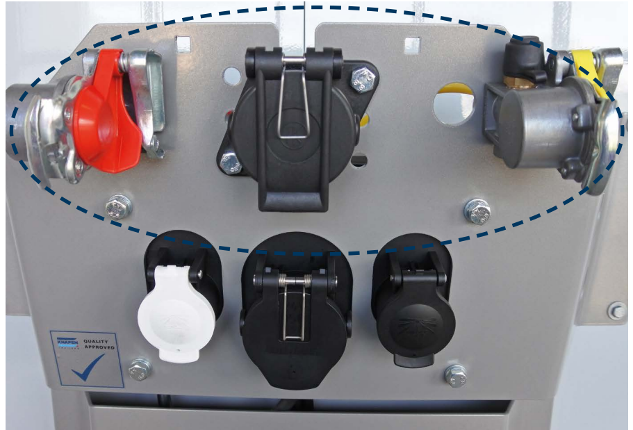
The connections for EBS modulator are located on the headboard of your trailer
