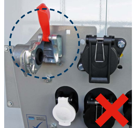
Always close the covers on the hose couplings so that no contaminants can enter the hoses
