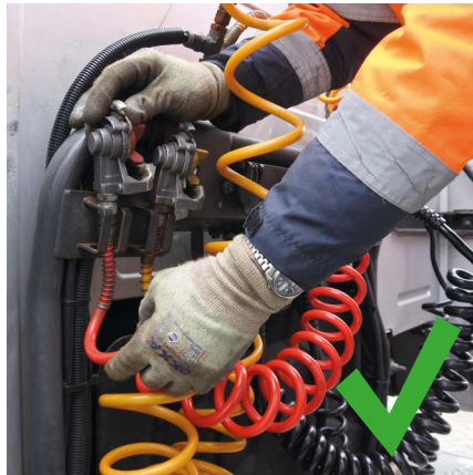
Tip: Suspend the air hoses from the truck after uncoupling.
