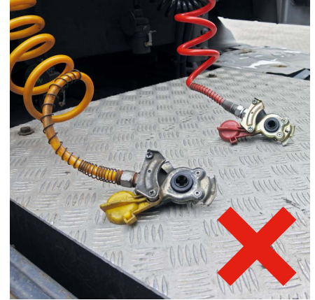
Always close the covers on the hose couplings so that no contaminants can enter the hoses
