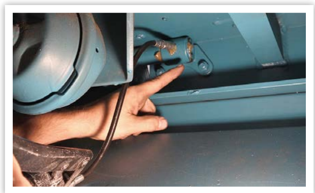
2. Grease the system with a grease gun
