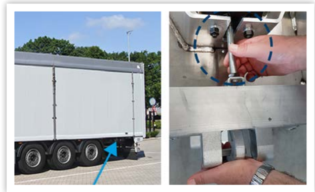
Adjust the position of the pneumatic rear door locking device with a rotating movement
