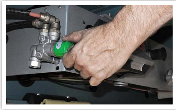
Step 3: Withdraw the green button on the control panel to release the pneumatic door locking device
