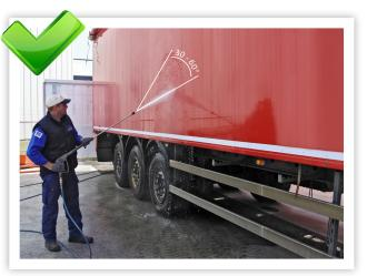
3. Start spraying from bottom to top for proper drainage of the dirt. Never spray into the joint seams. This way you avoid further penetration of dirt into the seams.
