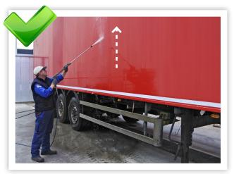
4. Do not use water pressure of more than 60 bar (870 psi). This prevents paint damage due to excessive water pressure per cm<sup>2</sup>.
