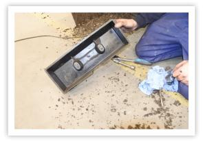
4. Unscrew the plug from the connector and then clean the plug, connector and the back plate thoroughly.
