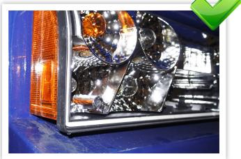
2. Put the light cover back in place. Make sure that it joins up correctly.
