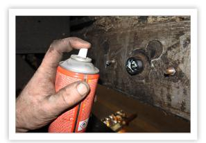
6. Reconnect the plug and reassemble the cover. Repeat this process for the cover at the other side of the trailer.
