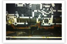
DIRT AND MOISTURE UNDER THE LIGHT COVER LEADS TO CORROSION,
