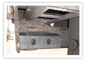
**Tip 2: Thoroughly check the seals of your lighting covers**Every light cover of the trailer has a rubber seal to protect the lights and the lighting plate behind them against moisture and dirt. Proper closure and sealing of the light covers are crucial for the lifespan of your lighting system.
